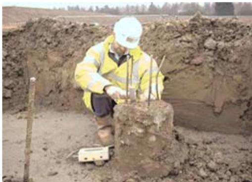
Pile Integrity Testing (PIT)
